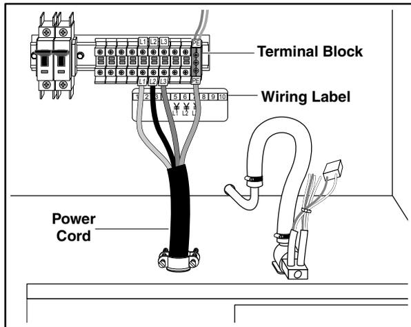
**Figure 5: Power Supply Cable Connection**
