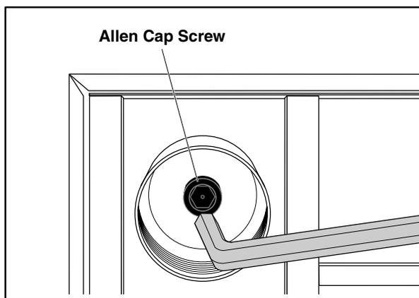
**Figure 2: Allen Cap Screw Location**
