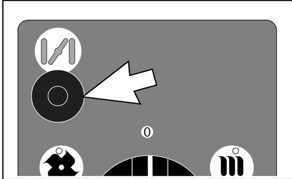
Figure 10: Oven Vent Valve
