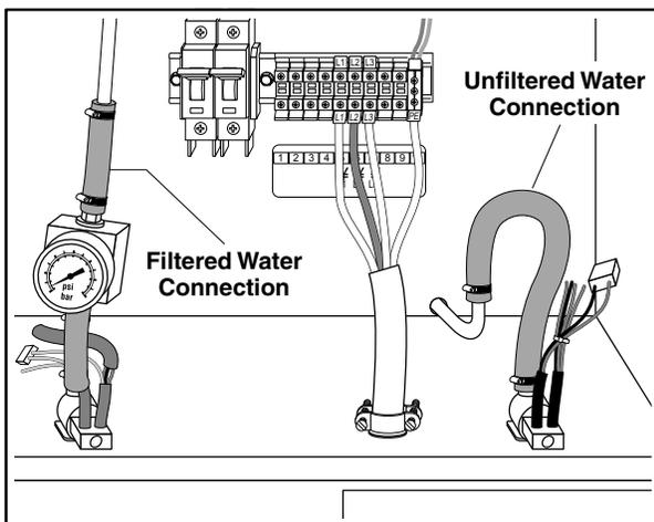
**Figure 7: Water Supply Connections for CEM20U**
