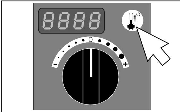
Figure 19: Oven Temperature Button
