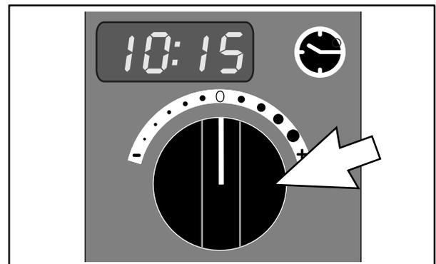
Figure 22: Oven Timer Adjustment Knob
