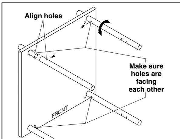
**Figure 3: Leg with Threaded Holes in Proper Position**
