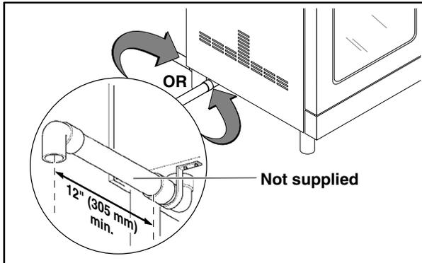
**Figure 8: Drain Connection**
